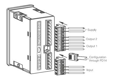
Fig. 3. View of controller connection strips
