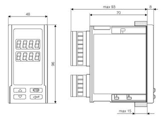
Fig. 2. Controller overall dimensions
