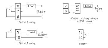
Fig. 5. Supply and load circuit connection
