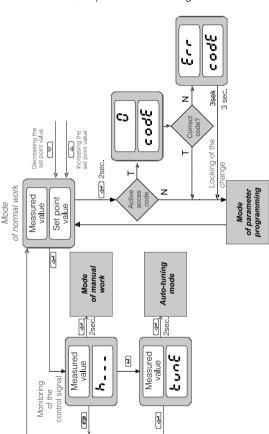
Rys. 7. Menu of controller service
